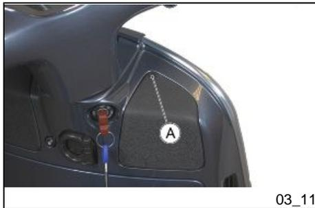
Check coolant when the engine is cold as indicated in the scheduled maintenance table, following the steps below.
